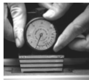
Correct alignment of needle to registration mark.
