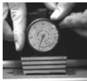
Incorrect alignment of needle to registration mark.
